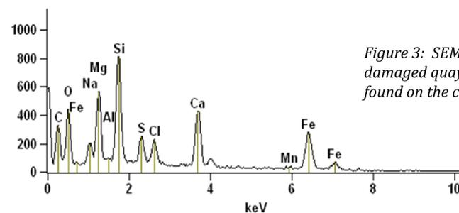
Figure 3: SEM-EDX results of metal coupon from the damaged quay wall structure. Sulfur was frequently found on the coupon surface.
