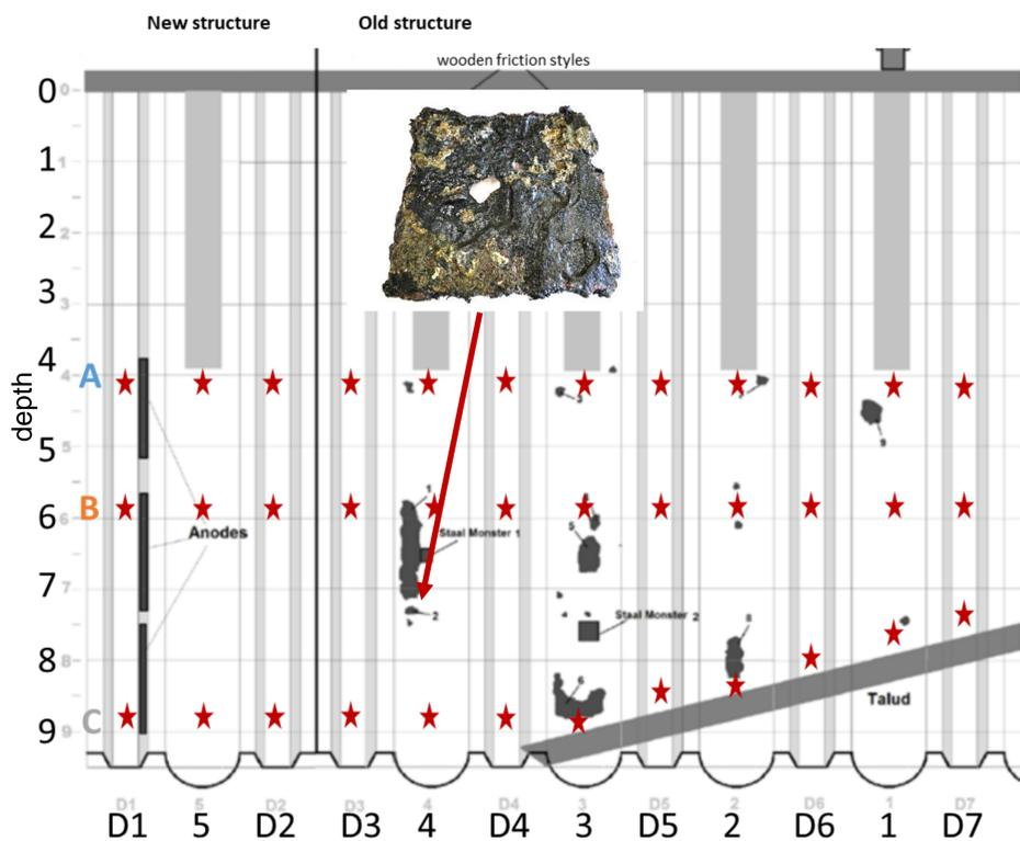
Figure 1: Overview of damaged quay wall. Red arrow shows location of sampled coupon taken out; red stars indicate locations for potential measurements and wall thickness measurements at different depths (A, B, C). Results of potential and wall thickness measurements are shown in the diagrams at the right.
