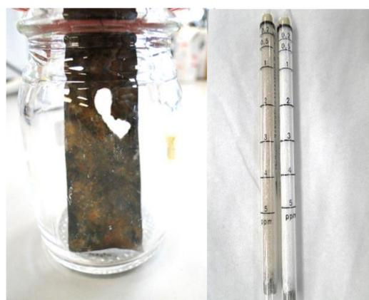
Figure 2: Volatile sulfide determination from corrosion product sample.
