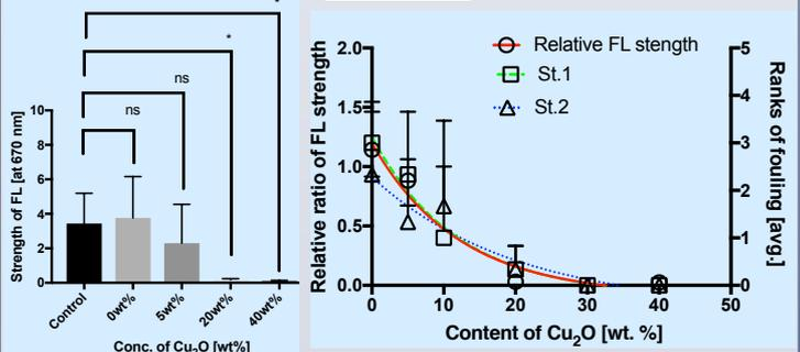
Figure 5. Relative comparison of experiment with control between  $\text{Cu}_2\text{O}$  content and the FL strength (left), relationship between relative FL strength vs ranks of fouling (right) (St.1: Hiroshima, Japan, St.2: Okayama, Japan)
